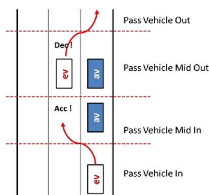
Fig. 4: Pass Vehicle Maneuvre
