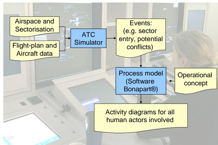
Fig. 2: Main components of the controller workload model
