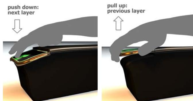
Picture 4: Pushing the touch paddle down to make a selection; pulling it up to go back to the top layer
